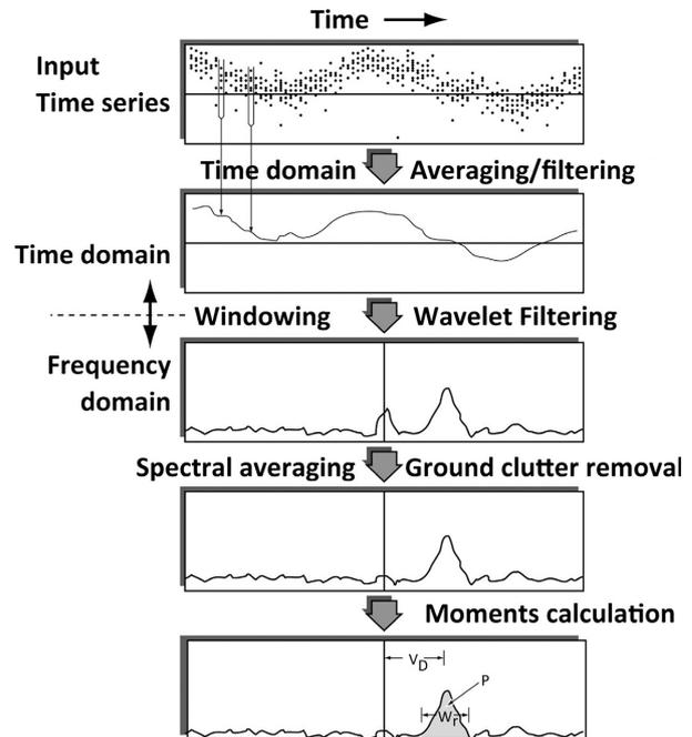
Fig. 4. Data processing: Moments estimation from I/Q time-series data (Vaisala 2007).
