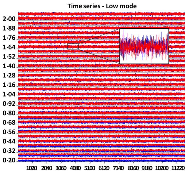
Fig. 3. Example of clear air in time series presented as normalized I/Q plots for each gate in low mode.
