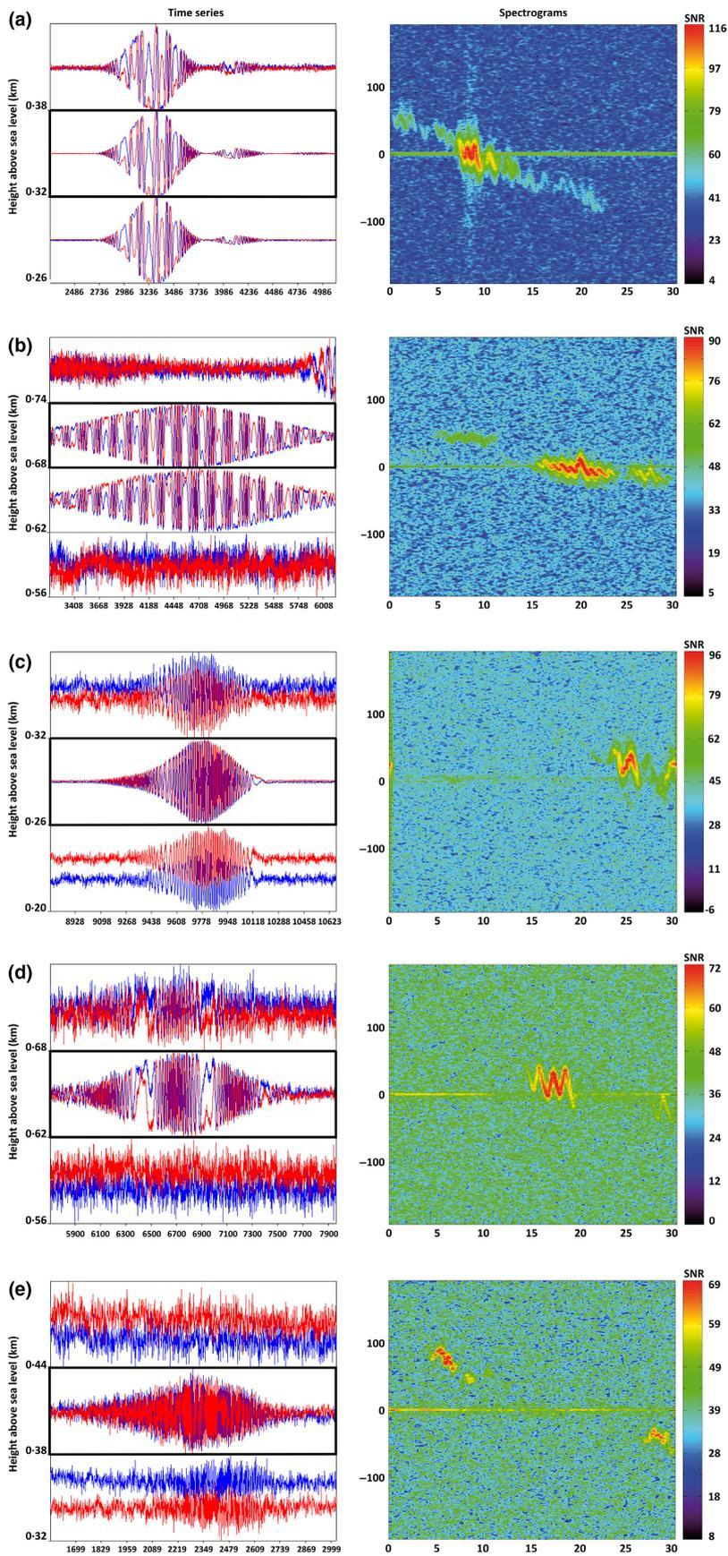
**Fig. 6.** Time-series (left) and spectrogram (right) plots for qualitative classification: (a) is 'very good' (15 March 2015, gate at 0.32 km), (b) is 'good through beam centre' (10 March 2015, gate at 0.68 km); (c) is 'good marginal' (17 March 2015, gate at 0.26 km); (d) is 'poor through beam centre' (17 March 2015, gate at 0.62 km) and (e) is 'poor marginal' (17 March 2015, gate at 0.38 km). The spectrograms show only the data from the single-range gate framed in the time-series plots.
