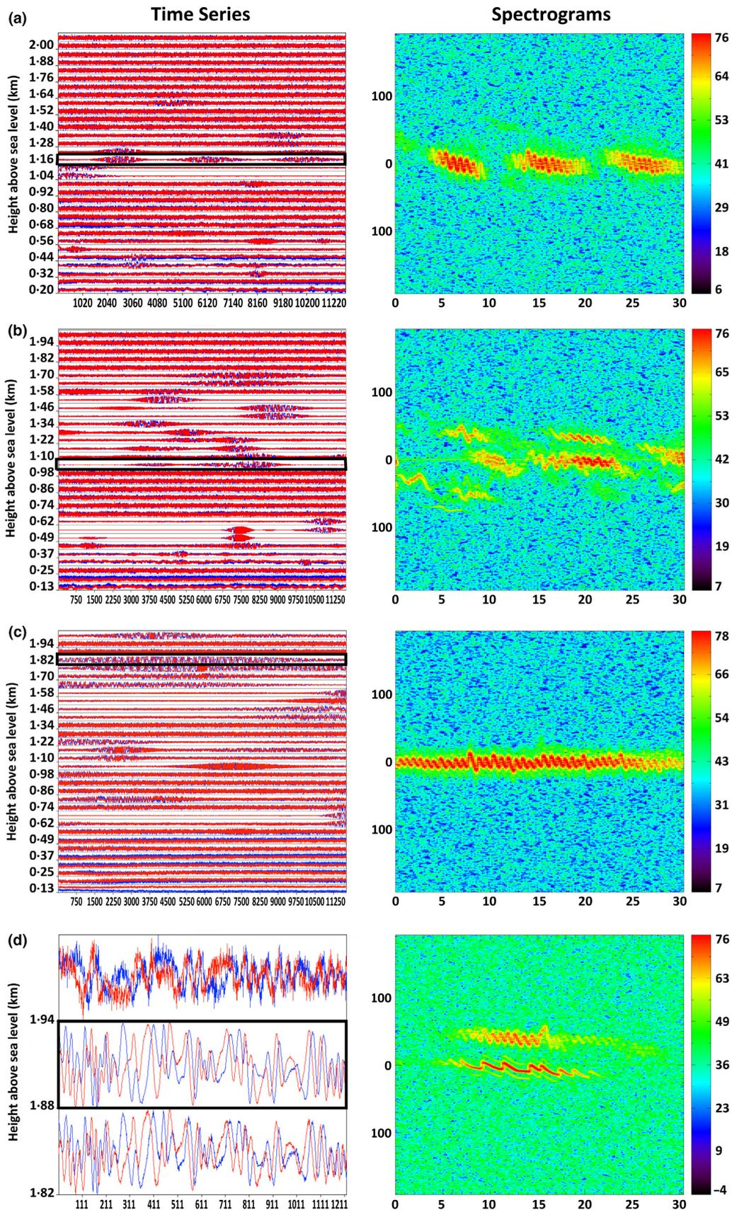
**Fig. 7.** Various examples of birds in time series and spectrograms on 30 March 2015. (a) Three different birds in the gate at 1.16 km; (b) high migration intensity, birds occurring simultaneously in the gate at 1.097 km; (c) long bird echo in the gate at 1.82 km and (d) overlapping echoes of two birds in the gate at 1.88 km. The spectrograms show only the data from the single-range gate framed in the time-series plots.
