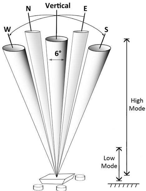
Fig. 2. Beam configuration of the boundary layer wind profiler radar at Punta Galea, Spain.
